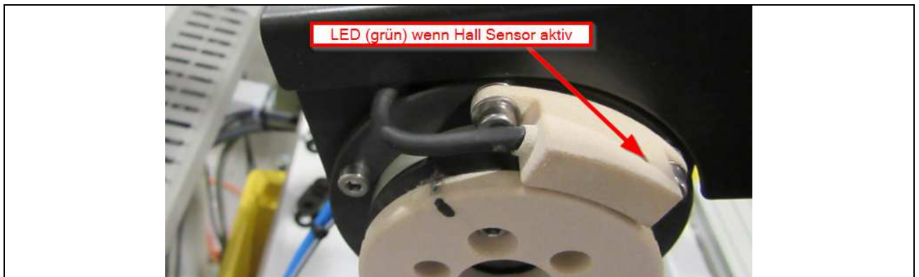
Pic. 4: Prototype assembly of the sensor with joint RL-D-20
